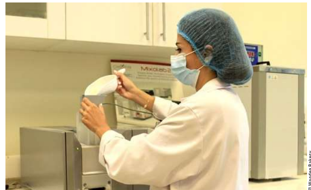
In minutes, the Mixolab 2 dough characterization tool can profile a flour sample's water absorption capacity, mixing behavior, and amylase activity
