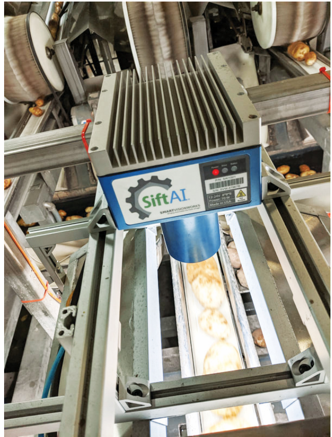
AI-driven sorting and grading systems, such as the SiftAI® Machine Vision System shown here, help potato packers improve processing throughput and accuracy while reducing labor costs.
